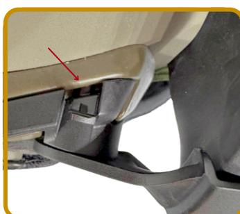
Place the visor clip in the rail notch slot at the top front of the rail. If the clip is sticking out like above, the visor is not completely mounted.
